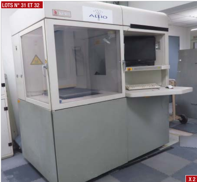
► Imprimante 3D par stéréolithographie 3D Systems, mod. SLA 5000, environ 15 000 heures (1998) ► 3D printer by stereolithography, 3D Systems, mod. SLA 5000, approximately 15,000 hours (1998)
