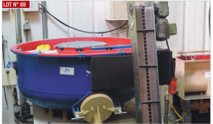
► Tribofinition Wheelabrator, type CD 300 (2005), volume de travail 300 litres, volume utile 160 litres ► Tribofinishing Wheelabrator, type CD 300 (2005), volume of working tank 300 litres, effective volume 160 litres
